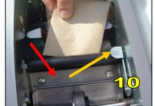
guide plate of the pan. NEVER use sharp tools or blades on the plates, that can be easily scratched and cause new jams...
