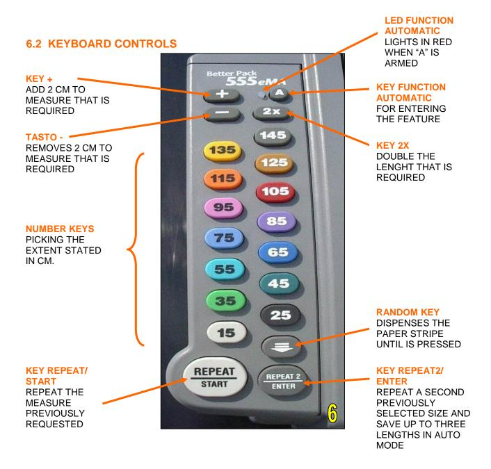
The colored buttons corresponding to the 14 listed measures, from 15 to 145 cm. The button "random" (the one with the arrow down) distributes the strip of paper until pressed. Some functions to help the operator are given by the devices and key combinations listed below. If any of this combination does not work, you should feel a "Beep". In this case, repeat the key combination.
