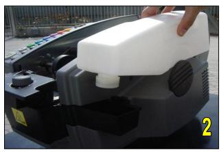
**5.2 MOISTENING OF THE BRUSHES:** to activate the system of moistening of the brushes, wash with hot soapy water before starting up, then mount them in the pan so that the side with greater height is in the front position (as seen in 1). By placing the bottle remains constant moistening.
