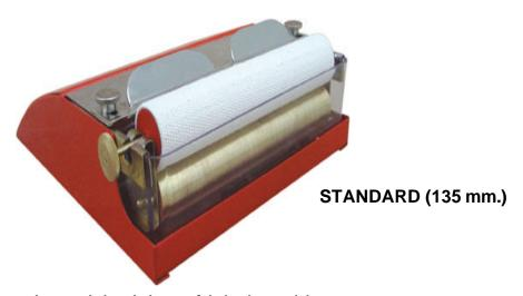
The STANDARD allows the quick gluing of labels, addresses etc. up to an opening width of 135 mm. Simply run the item which is to be glued over the fabric finish roll. The film of glue, which is constantly replenished as the rollers turn, enables you to obtain ain perfect gluing of the whole surface. Built in plastic and stainless steel. For bigger widths we recommend the DIN A/4a ( 210 mm) e SONDER (280 e 360 mm) with same functional features and built in nickel-chromium steel.
